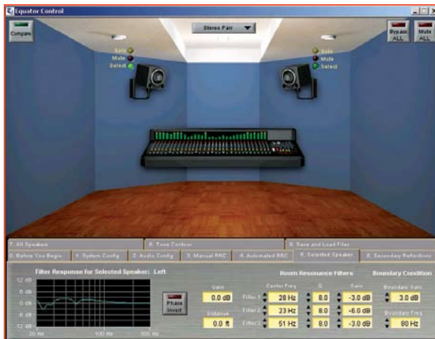
The Equator Control software calculates primary room modes and then instructs the monitors how to correct for room anomalies.
